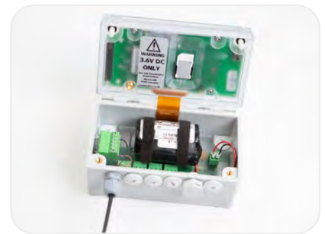
Insert connector into plug in terminal connector.
