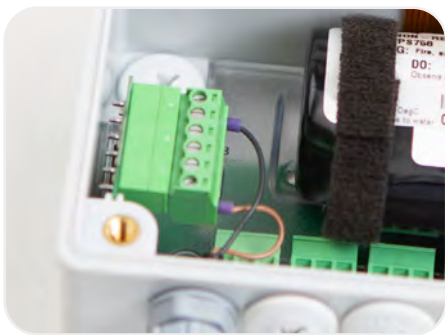
Insert card into Ex socket.
