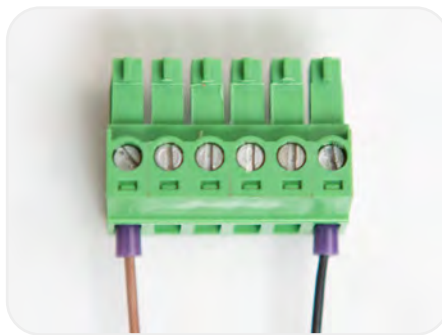
Wire in to green connector plug and tighten screw.
