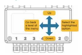
Press any button to wake the Metron4. Press left to cycle channels for immediate reading (config. dependent) or enter PIN (1234) and press right after 4<sup>th</sup> digit to enter homepage.
