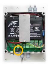
Ensure the highlighted switch is positioned at Solar.
