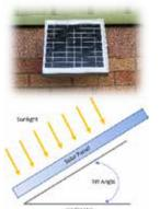
Solar panel comes attached to a mounting bracket. The panel must face directly south and have a view of at least 100° of unobstructed sky.
