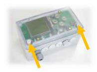
Place unit on a flat surface and loosen the 2 nylon screws in bottom corners to open.
