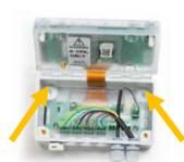
Use the 2 mounting holes to screw the Metron4 down onto a flat surface.
