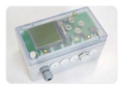
Place the unit on a flat surface and loosen the 2 nylon screws in the bottom corners to open. Allen key required.
