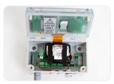
Open the Metron. The interior will vary depending on unit. The image shows the /SSM model with a battery.
