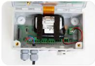
Plug the connector into the correct input channel and tighten the gland. Ensure cable is through the gland. Plug in the power source.
