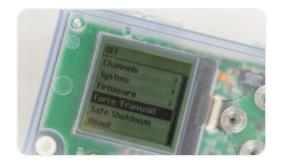
Force transmit. Move down to Force Transmit, and right to select. Watch the progress bar and wait for the unit to transmit. Once complete, the data will be available for viewing on MetronView. The unit will countdown for 40 seconds then enter Run Mode. The screen will turn off.
